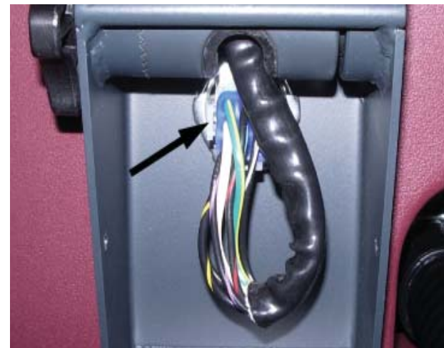
7. The wire harness must be aligned with the patterns on the connector to fit.
